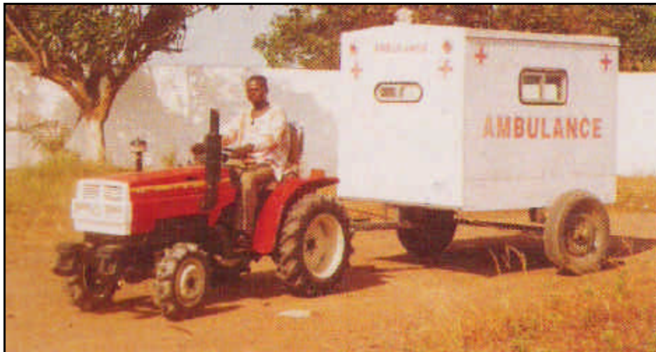
The tractor-driven ambulance- one of the new vehicles, tested by the Ghana Health Service – its impact to be evaluated by ITDP (photo: GHS / not shown: Indian Baja-Tricycle)
